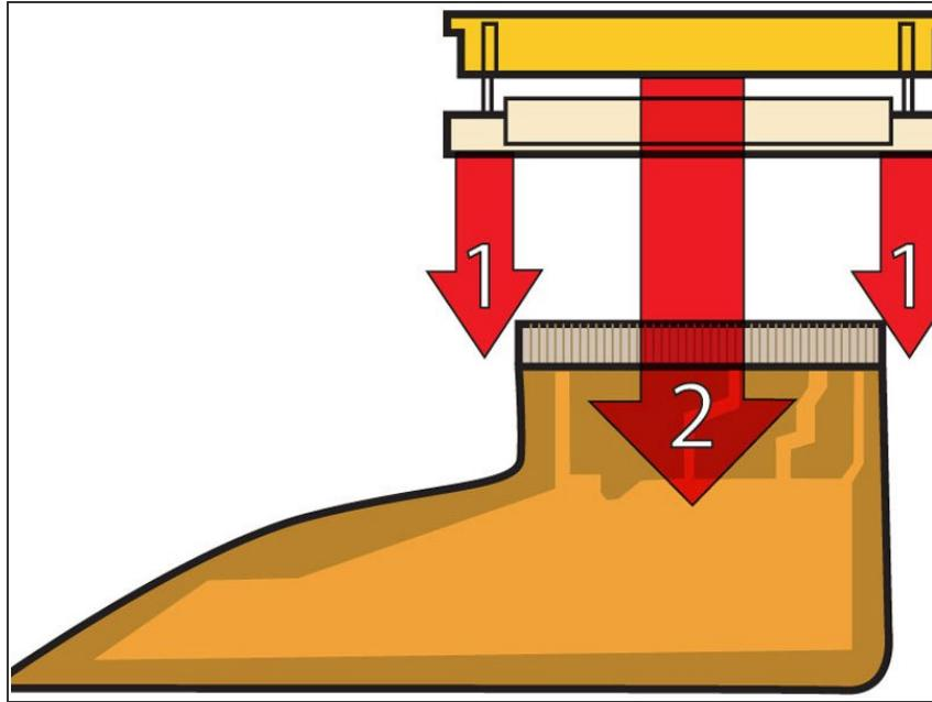
*(i)* This is a diagram of the ribbon clamp connector you will disconnect in the next step.
